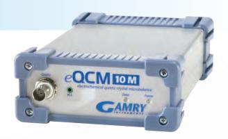
sensor binding events are all interfacial processes that produce mass changes. These mass changes can be measured by monitoring the resonant frequencies of an oscillating quartz crystal.
