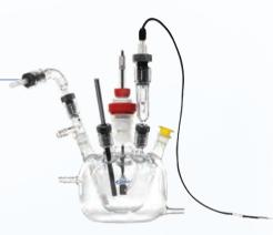
Hg/Hg<sub>2</sub>SO<sub>4</sub> reference electrodes (electrodes ordered separately), one Ace-Thread port for a counter electrode, one 14/20 ground glass port for inert gas purging/blanketing (an adapter is supplied), one 14/20 ground glass port usable for temperature sensing, reagent addition, gas venting, etc.
